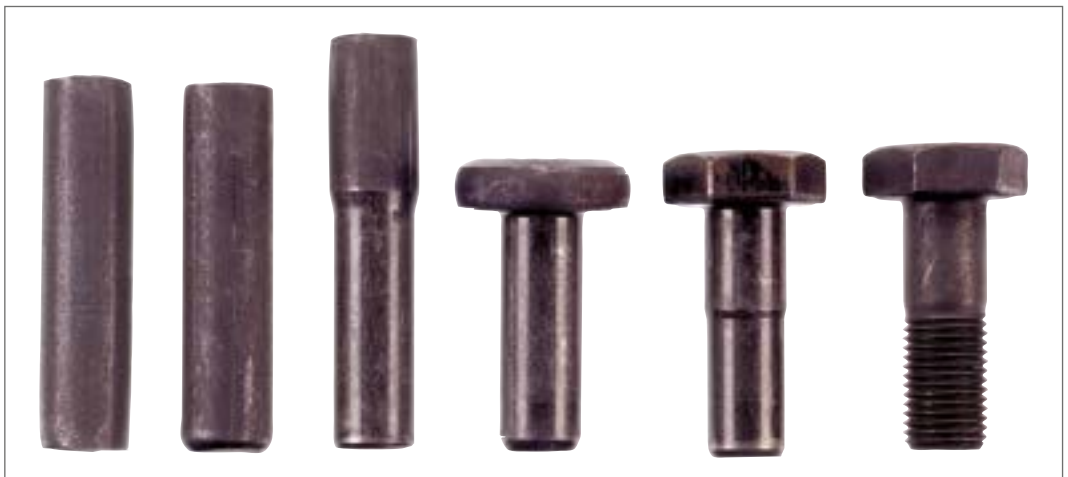
Figure 5.3 Forming stages of a hexagon head screw
